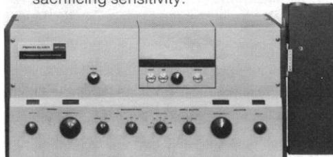
**A new ultra-micro flow cell accessory** with 20  $\mu$ l sample capacity converts the MPF-44A into an extremely sensitive, versatile LC detector. Other accessories let you select TLC, low temperature luminescence (phosphorescence), polarization, and solid sampling (front surface viewing).
