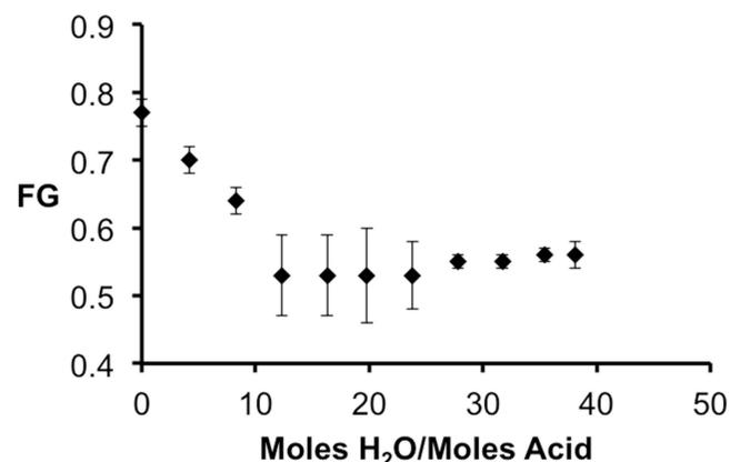
Figure 7: Relationship between fraction of gauche conformers and moles of H<sub>2</sub>O
