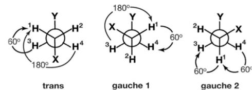
Figure 3: Generic gauche and trans conformers
